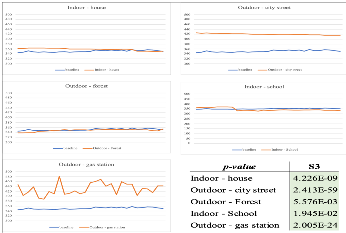
Fig 3: Plot data of the measurements recorded for butane, propane, methane, and gasoline at the different locations tested. X-axes represent the different measurements taken over time at that specific location. Y-axes represents the parts per million of hydrocarbons detected by the sensor. The table shows the p-values for each location compared to baseline. P-values \geq 0.05 are considered non-significant and are highlighted in red; p-values < 0.05 are considered significant and are highlighted in green.
