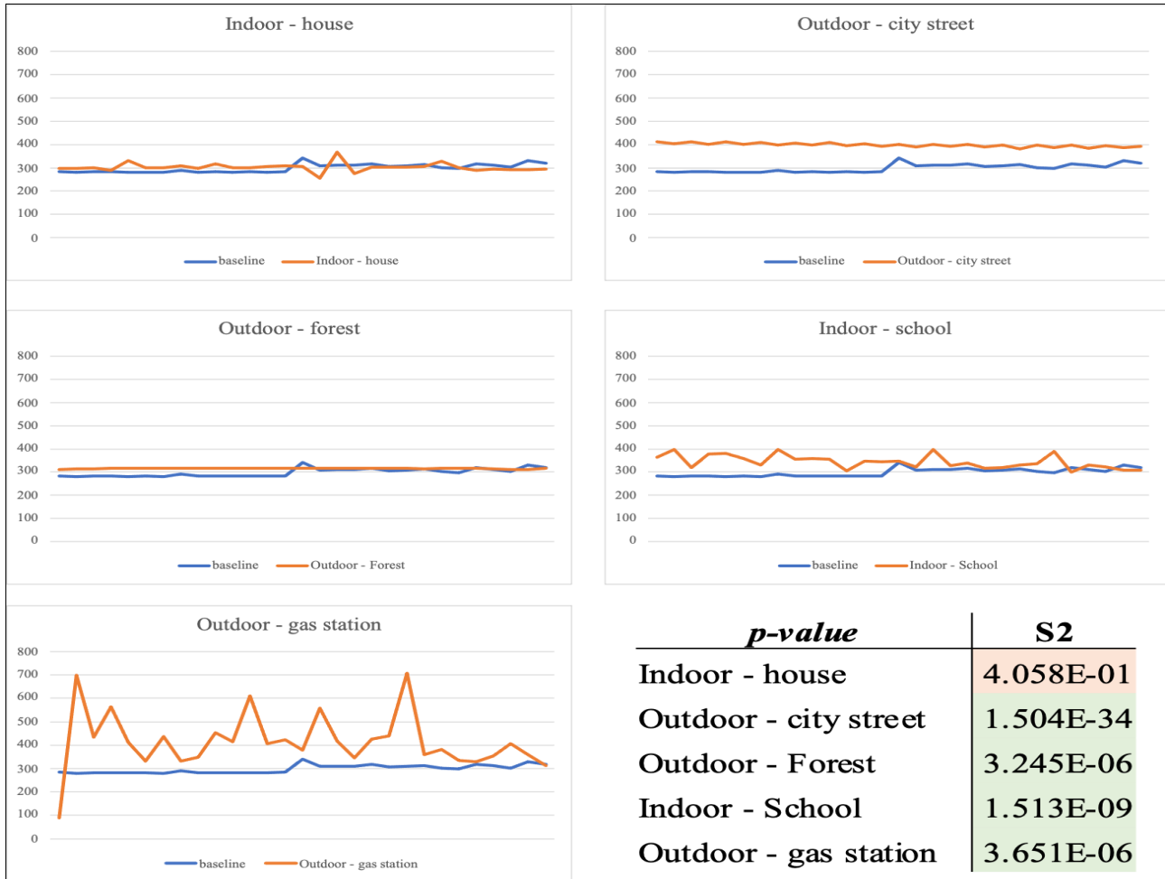
Fig 4: Plot data of the measurements recorded for carbon monoxide at the different locations tested. X-axes represent the different measurements taken over time at that specific location. Y-axes represents the parts per million of carbon monoxide detected by the sensor. The table shows the p-values for each location compared to baseline. P-values \geq 0.05 are considered non-significant and are highlighted in red; p-values < 0.05 are considered significant and are highlighted in green.
